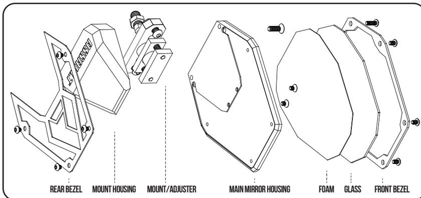
REAR BEZEL MOUNT HOUSING MOUNT/ADJUSTER MAIN MIRROR HOUSING FOAM GLASS FRONT BEZEL
